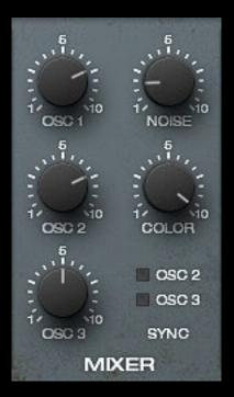
Inside the Mixer section, the volume control for all three oscillators can be found. Next to the additional noise oscillator and it's own tone filter.
