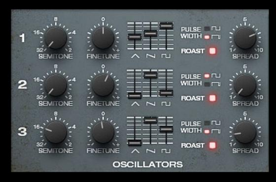
The oscillator section contains 3 oscillators, each of them generates 3 waveforms at once: triangle, sawtooth, pulse (with 50% or 90% pulsewidth).
