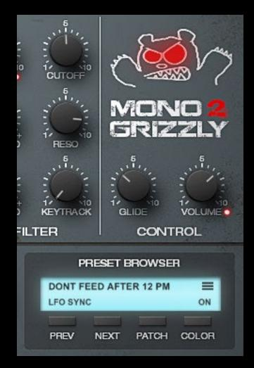
On the right side of the MonoGrizzly you have access to the preset browser. Here you can step through the presets by using "Prev" & "Next". By clicking on the 4-line symbol the preset list will show up. You can also rename presets with right-mouse-click on the preset name. The button "Patch" opens the menu for loading and saving single presets and preset-bank.
